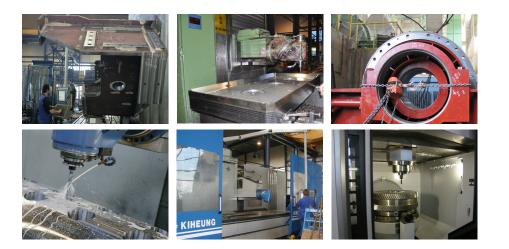
2x CNC Bed type milling machine 5 mtr Length 5000 mm Width 1200 mm Height 1500 mm
