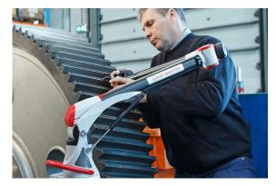
**On-site 3D gear measurement arm**
